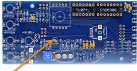
**NOTE!** Ensure the flat face on the component matches the flat face on the PCB silkscreen. You need to bend the middle lead of the component backwards to achieve this to go through the centre hole. Orientation is vital.
