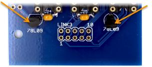
**NOTE!** Ensure the flat faces on the components match the flat faces on the PCB silkscreen. You need to bend the middle lead of the component backwards to achieve this to go through the centre hole. Orientation is vital.
